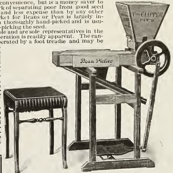
The "Clipper" Foot-Tread Pea and Bean Picking and Sorting Table.
