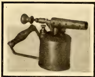
Soldering-iron Blast Lamp Using Spirit
