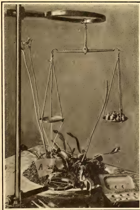
☞ Manner of ascertaining pressure exerted by Trap at A, while digesting a fly. Weight required to pull trap open as shown was about 80 grams (the weight of three silver dollars). Trap at B is open after several days' work in digesting a fly.
