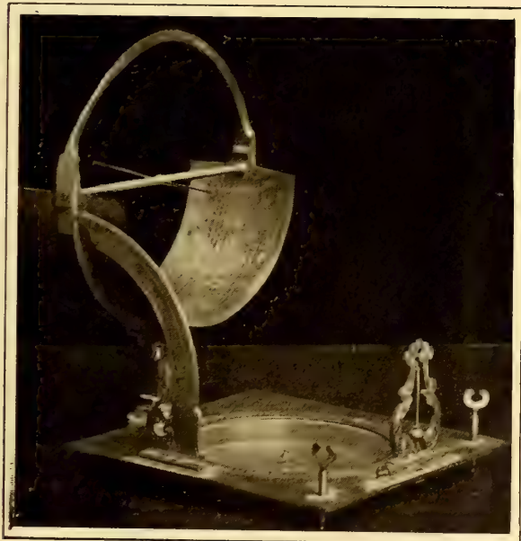
A Brass Sun-dial with Plumbob for Leveling
