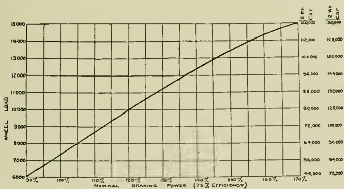
Fig. 2—Relative Braking Power Required for Cars of Different Weights to Produce the Same Retarding Force or Length of Stop.
