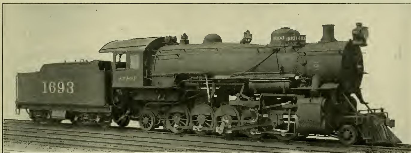
Powerful Simple Freight Locomotive of the 2-10-2 Type for the Santa Fe.
