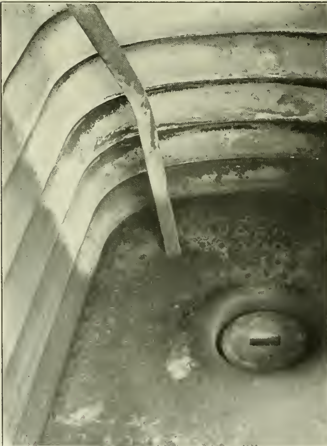
Back End of the Jacobs-Shupert Firebox After the Test.
