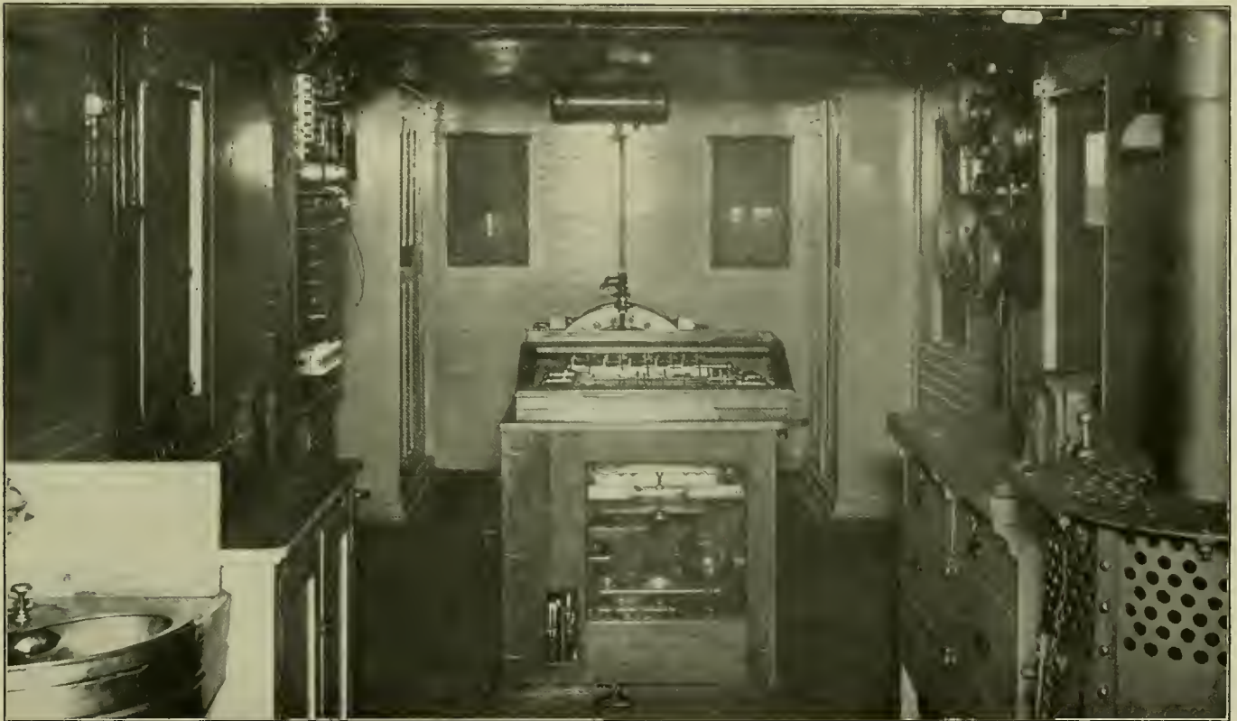
Interior View of Dynamometer Car, Showing Recording and Other Apparatus.
