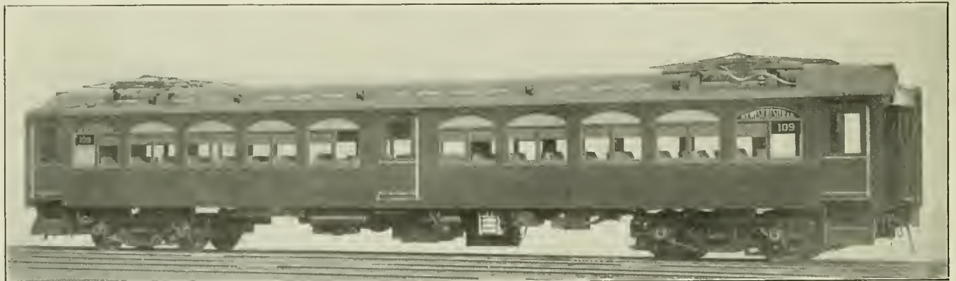
All-Steel Suburban Electric Car in Which Pressed Steel Shapes are Liberally Used.
