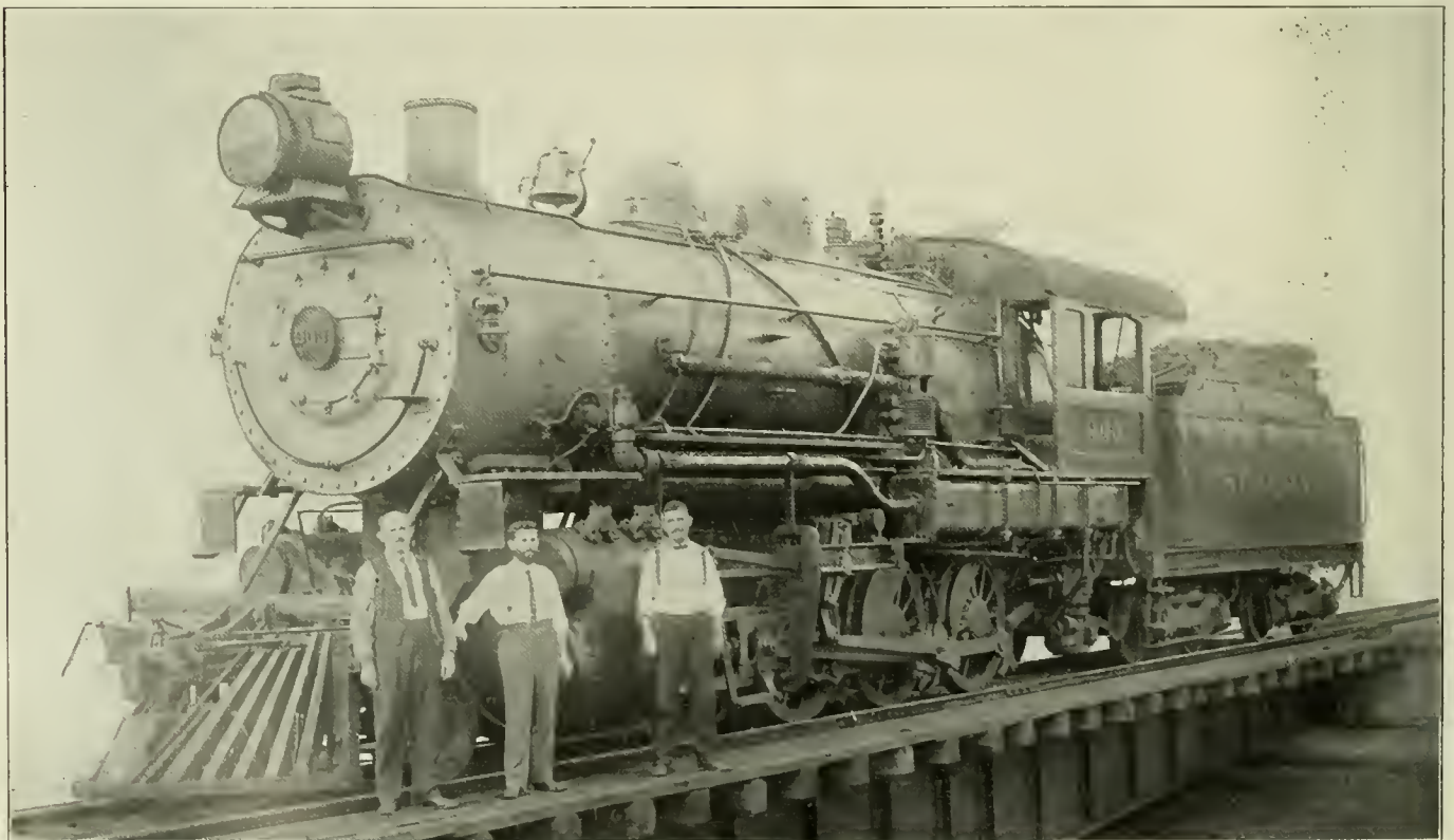
Consolidation Locomotive on the Seaboard Air Line Fitted with a Feed Water Heater.
