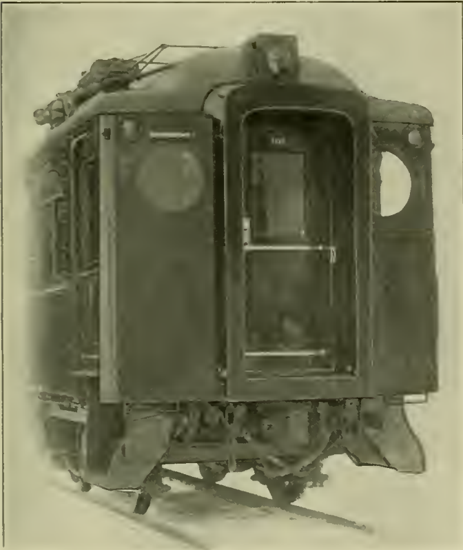
Vestibule of All-Steel Suburban Car.
