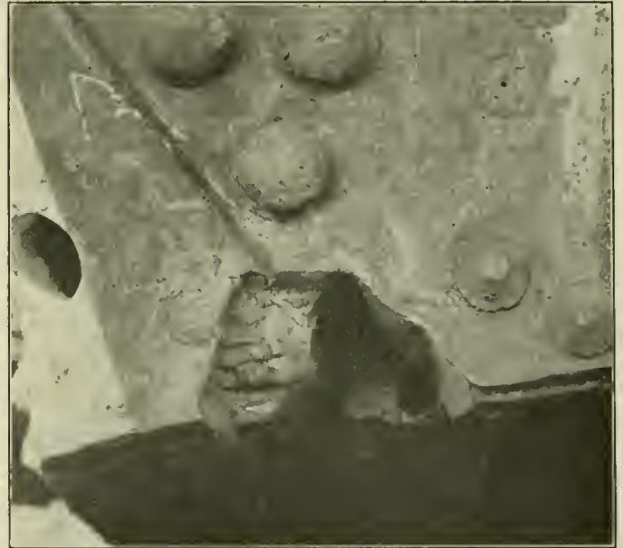
Fig. 2—It Was Necessary to Remove More of the Defective Mud Ring After Being Partially Welded.
