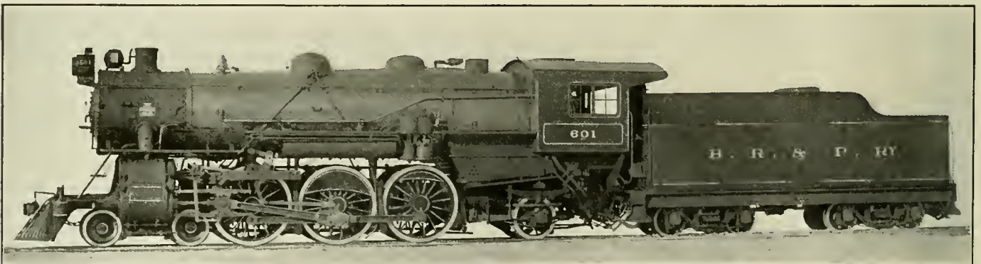
Locomotive Designed to Maintain 30 Miles Per Hour on a 1.5 Per Cent. Grade With a 400-Ton Train.
