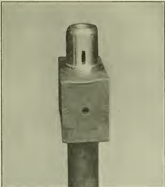
Fig. 13—Welded Valve Rod Guide Ready for Service.
