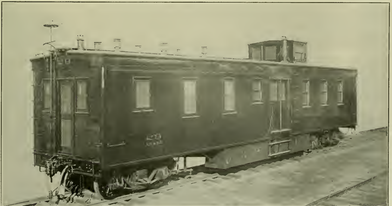
Dynamometer Car of 1,000,000 Lbs. Capacity; Atchison, Topeka & Santa Fe.
