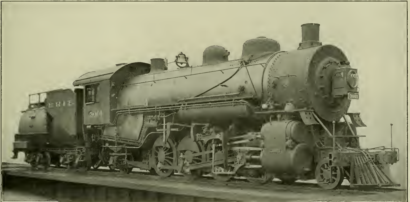
Powerful Mikado Locomotive with Superheater and Pilliod Valve Gear; Erie Railroad.
