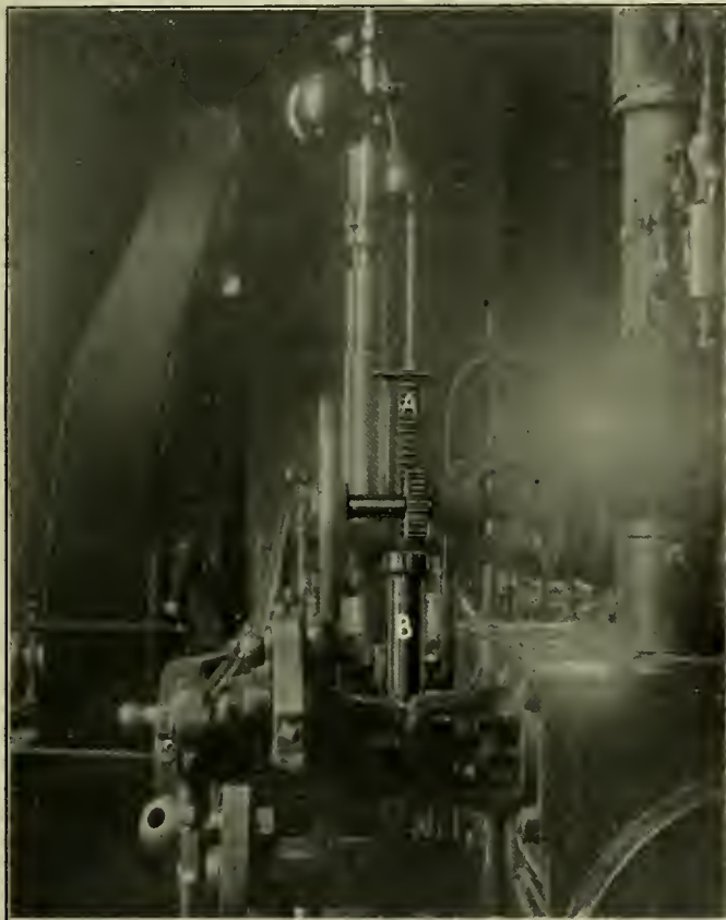
Fig. 5—A Simple Device, Controlled from Several Points In the Shop, for Stopping the Engine.
