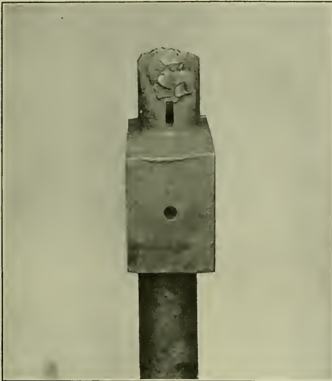
Fig. 12—Valve Rod Guide After Welding.
