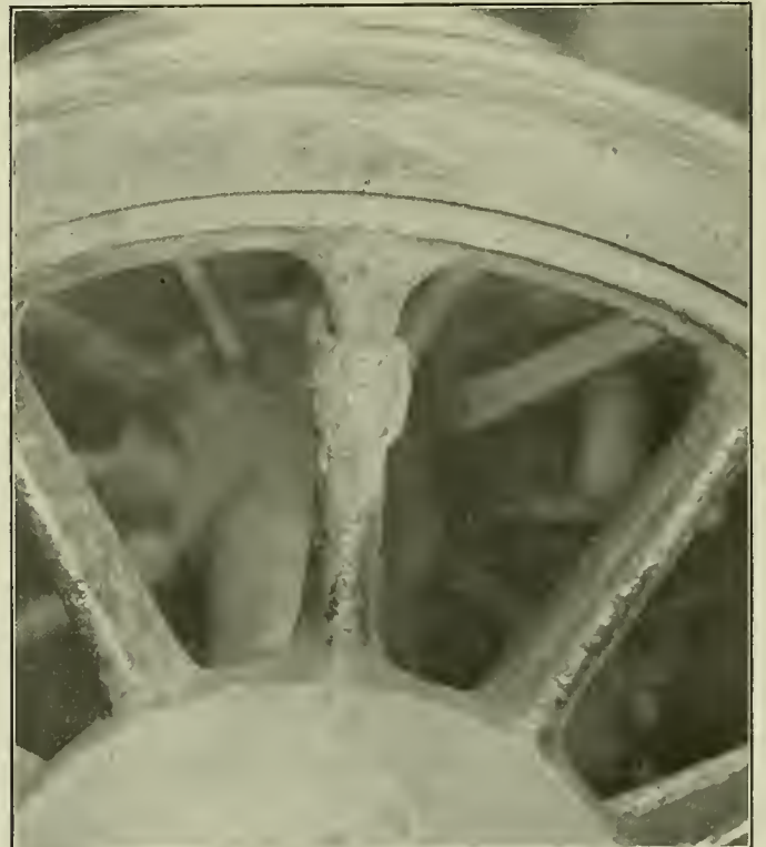
Fig. 15—Trailer Wheel Spoke Welded But Not Dressed.
