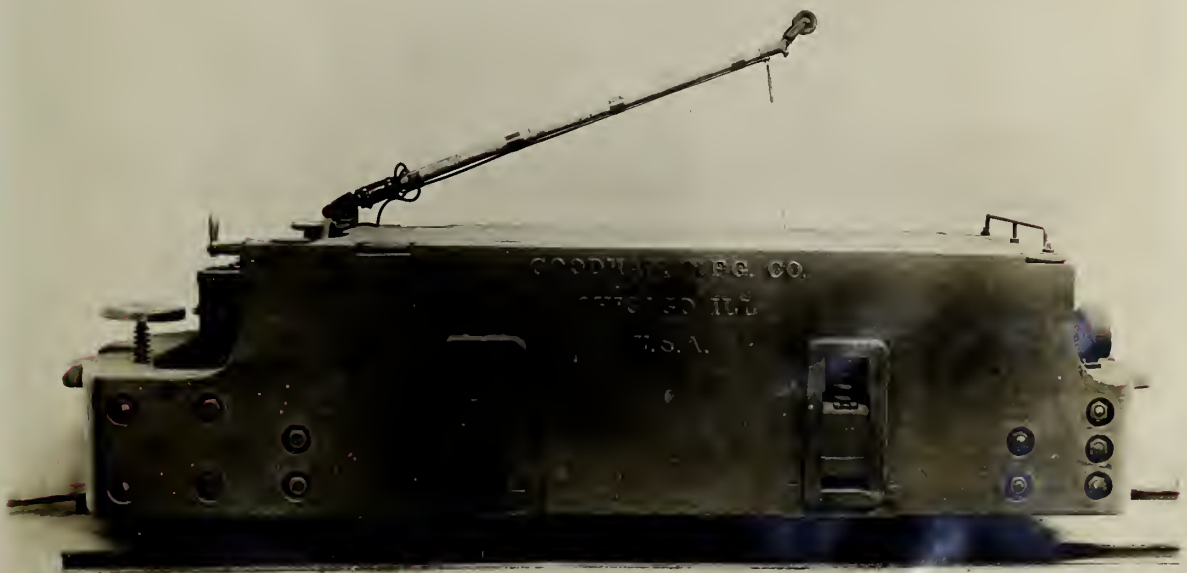
Goodman twelve ton (12-C-2) Two Motor Traction locomotive for gauges 36" to 48" Drive wheels 36" Wheel-base 48" Height about 44" Width 59 to 71" Length 12' 9"
