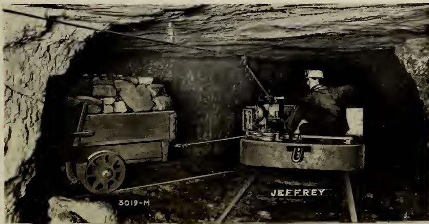
Rear View—Showing the Crab Device Pulling a Loaded Car from a Room.
