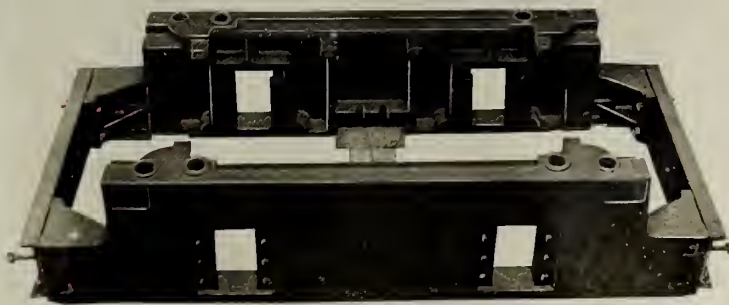
CAST FRAME WITH CHANNEL ENDS
