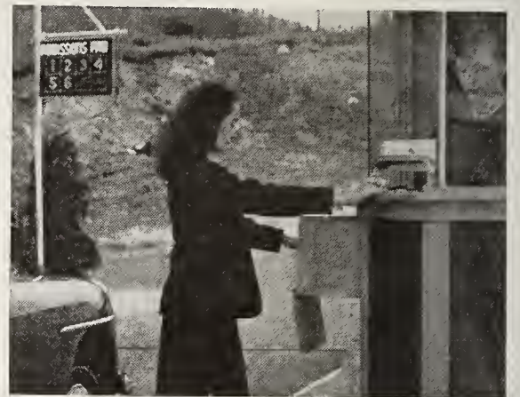
Sign at side of entrance lane registers number pressed by ticket seller, and car trips it off when it subsequently enters the theatre.
