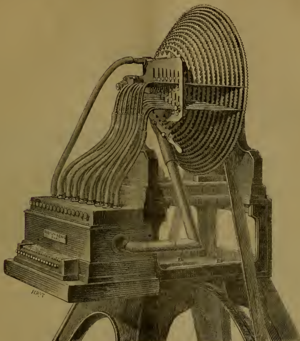
FIG. 5.—Koenig's Wave-disk Apparatus for synthetic researches on the quality of compound tones.
