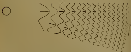
FIG. 6.—Positions of the slits in front of the wave-disks for combining the sounds with phase-difference \frac{1}{4} .
