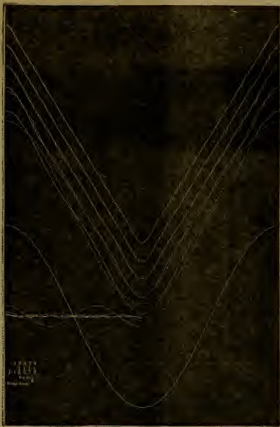
FIG. 3.—Resultant wave-form for odd members of series of upper partial tones when the difference of phase is a \frac{1}{4} .
