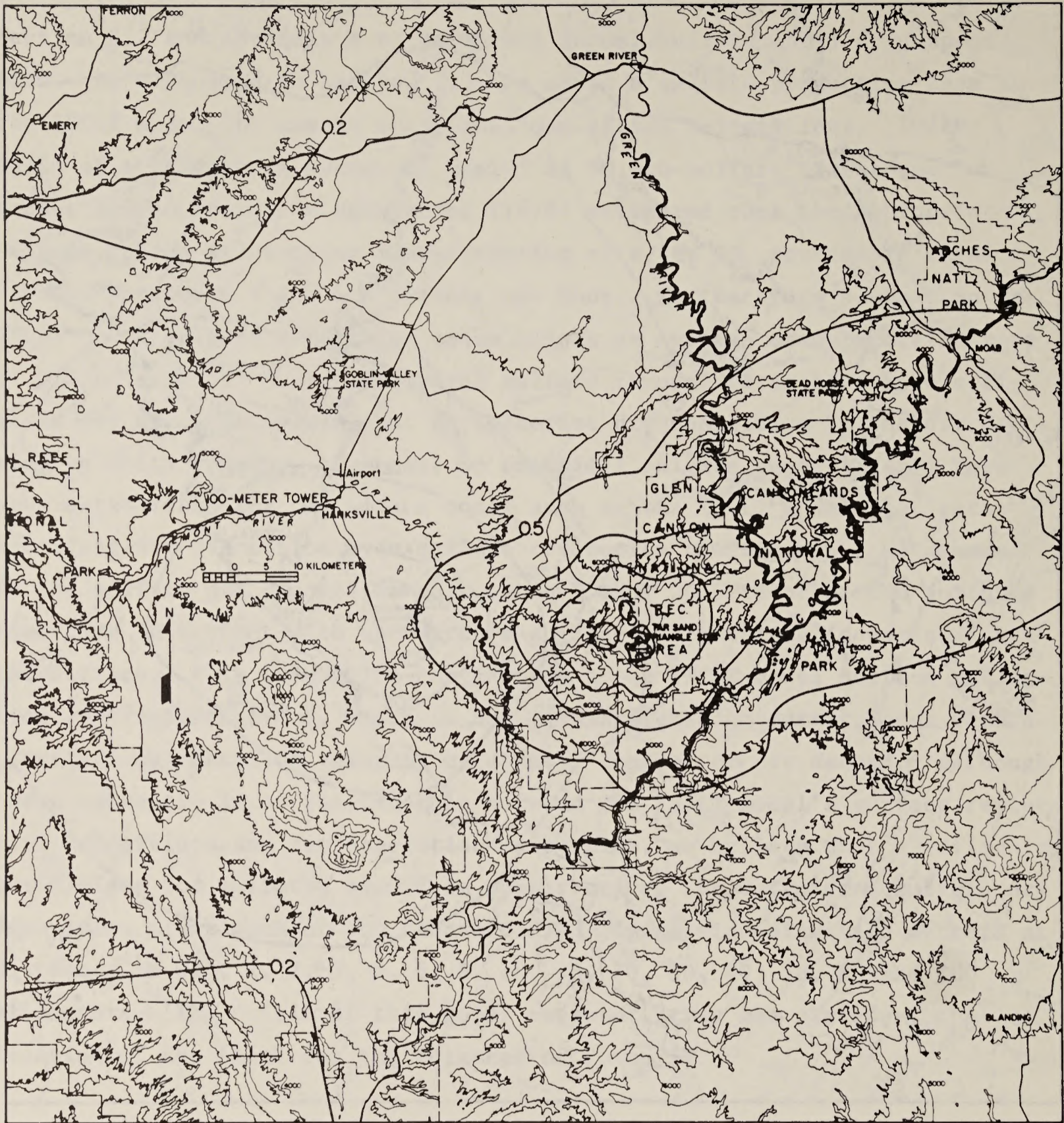
Figure 3-8. Calculated isopleths of annual sulfate dry deposition in milligrams per square meter attributable to the SO 2 emissions from Phase IV of the proposed Tar Sand Triangle Project. (One milligram per square meter is equal to 10 -2 kilograms per hectare.)
