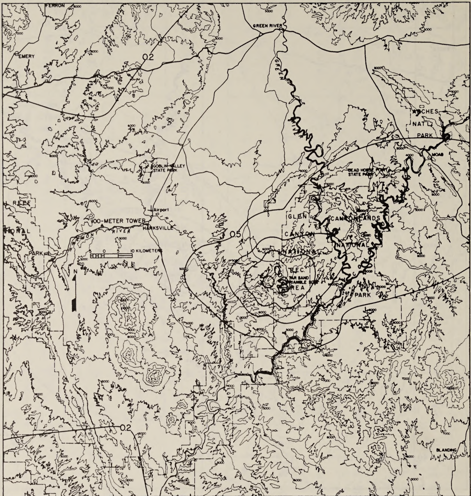
Figure III. Calculated isopleths of annual sulfate dry deposition in milligrams per square meter attributable to the \text{SO}_2 emissions from Phase IV of the proposed Tar Sand Triangle Project. (One milligram per square meter is equal to 10^{-2} kilograms per hectare.)
