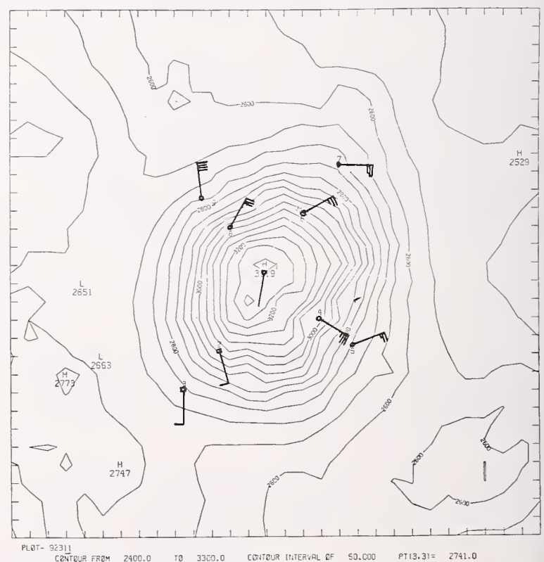
Figure 1a.--Airflow pattern measured by RAWS in the vicinity of San Antonio Mountain on September 17, 1981. Upslope draft--very light low aloft. Full barb is 2 mi/h (1 m/s), half barb is 1 mi/h (0.5 m/s), and a pennant is 11 mi/h (5 m/s).
