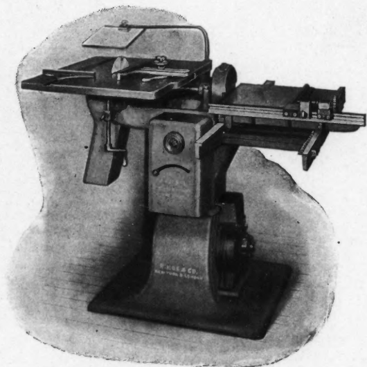
Combined Saw-Table and Trimming Machine (with electric motor)
