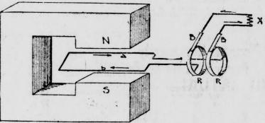
Production of Alternating emf. by revolving coil RR - Collector rings MS - Field magnet ab - Loop of wire DD - Brushes
