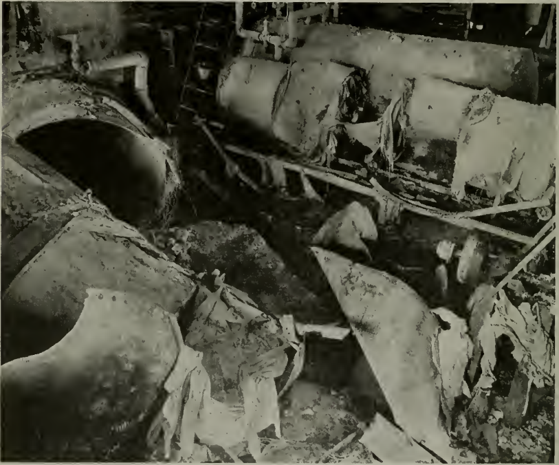
Figure 4—When a badly corroded vulcanizer exploded in a Pennsylvania plant, two persons were injured and the property damage amounted to $6,000. This shows parts of the exploded vessel.
