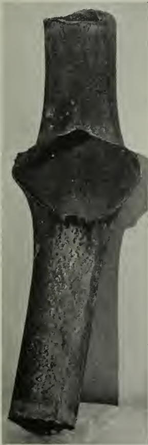
Figure 1—A close-up of the tube which signalled the difficulty illustrated in Figure 3. The rupture is 7" across.
