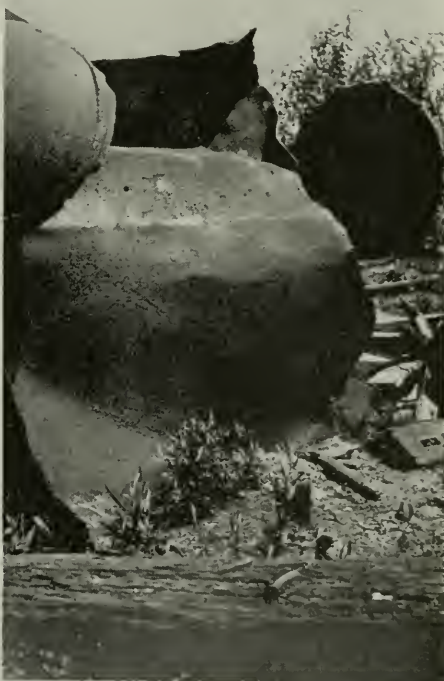
Figure 3. This uninsured air tank failure was traced by the inspector to lack of fusion in the welded longitudinal seam. The blast blew out a cement foundation and the air compressor and motor were hurled against the ceiling of the service station where the tank was used.
