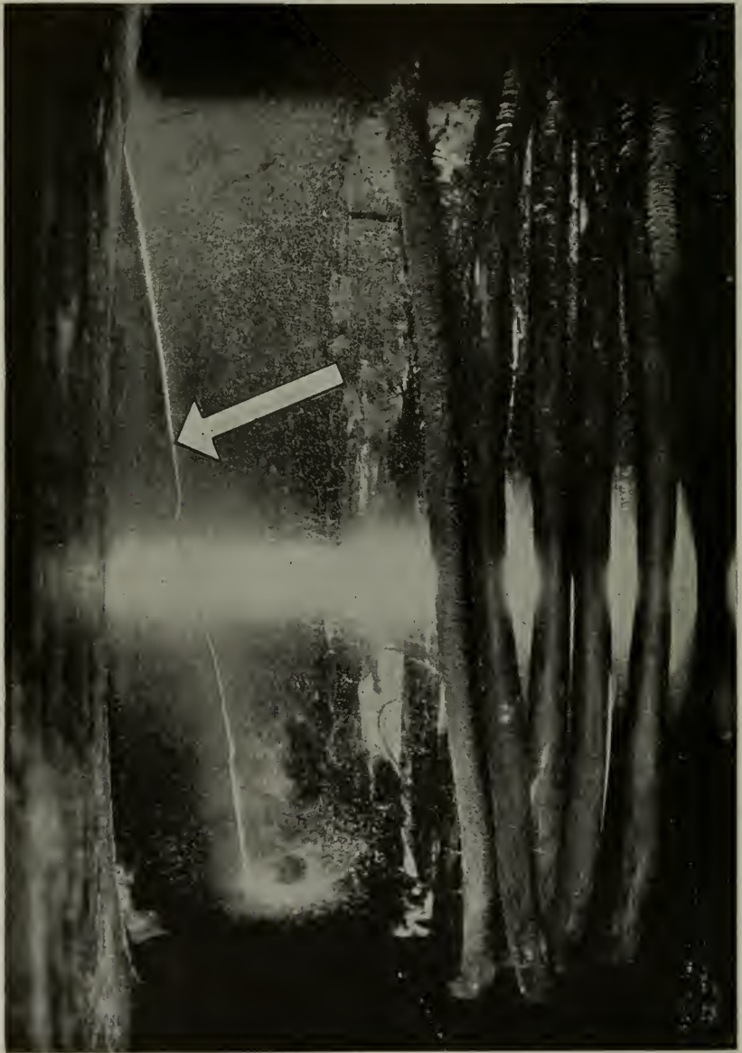
Figure 5—Magnaflux method applied to a shaft to determine the extent of a crack which had been detected by means of the unaided eye. The magnetizing coils are shown at the right.
