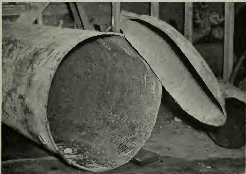
Figure 2—The tank which failed. The reversed minus head is clearly shown.
