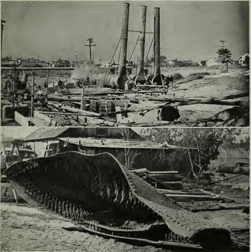
Figure 2—Above—An oil field drilling scene. Below—Outside wrapper sheet of the fourth boiler after it had traveled 900 feet.
