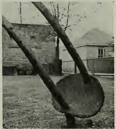
Figure 1—Head from a refrigerating vessel which failed at 150 lb pressure when the welded head seam gave way.
