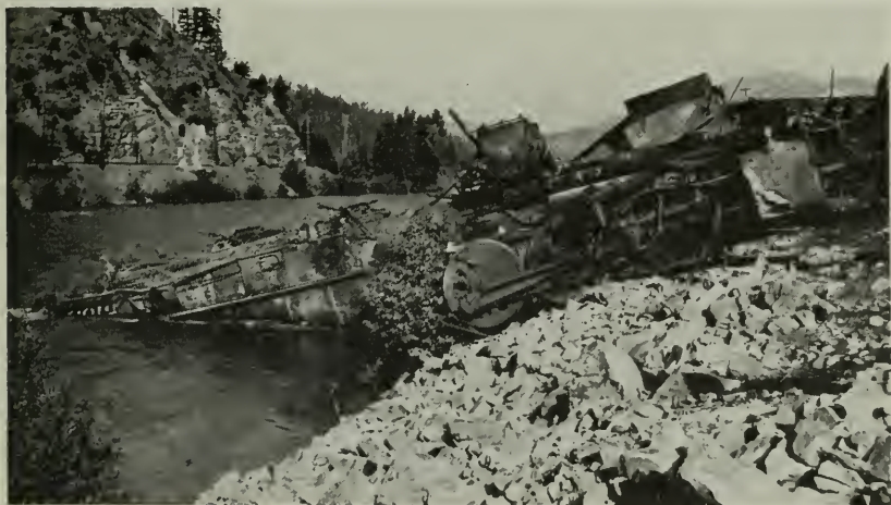
Figure 1—300 tons of locomotive toppled into a Montana river by the explosion of the boiler.
