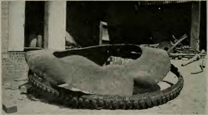
Head and seam of rendering tank which exploded after serious thinning because of external corrosion
