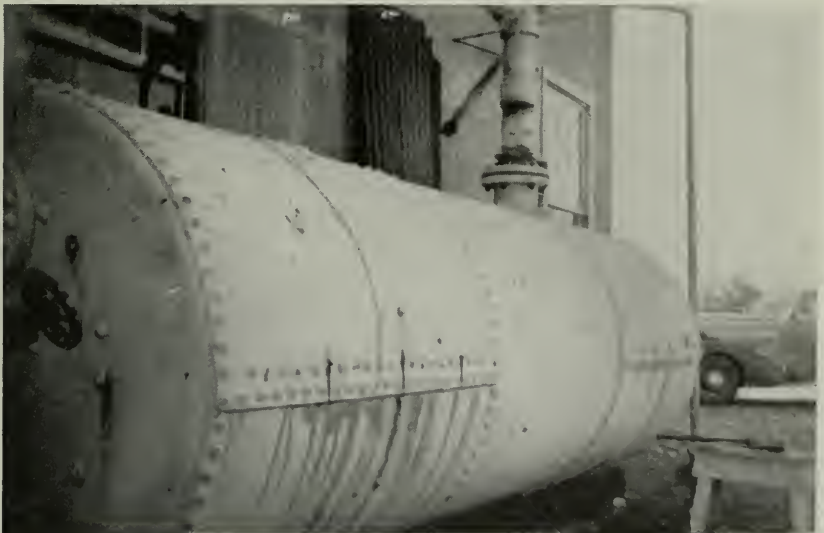
Possible explosion of this air tank was averted when hidden cracks were found by slotting the seams.
