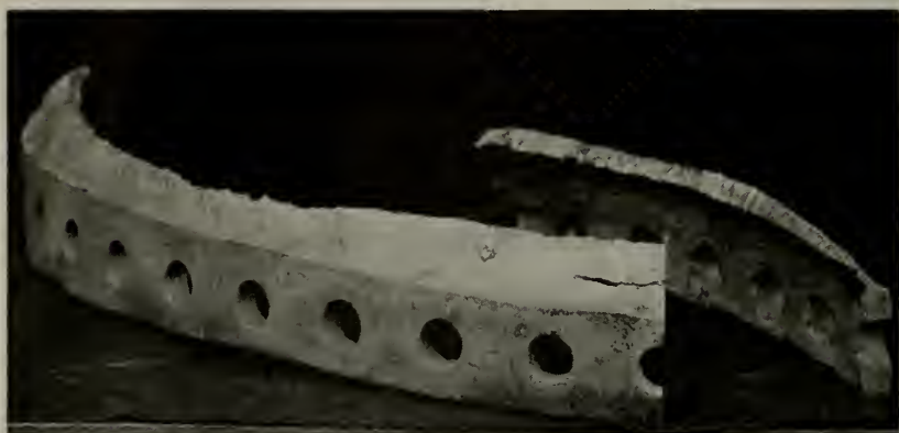
Figure 6—Parts of the lower drum of a water tube boiler showing the manner external corrosion wastes away the metal and weakens the head.
