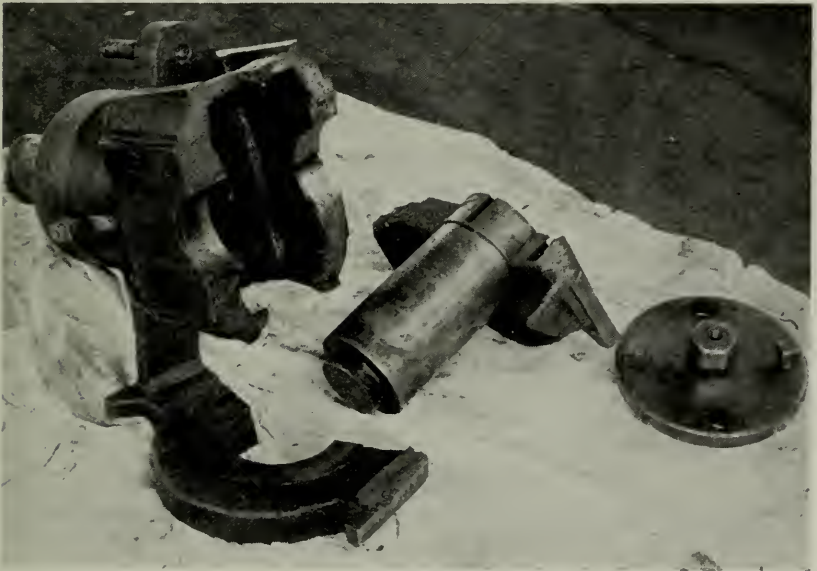
Figure 1—Broken parts following the failure of a cast iron crosshead. A dismantled inspection probably would have prevented this accident.
