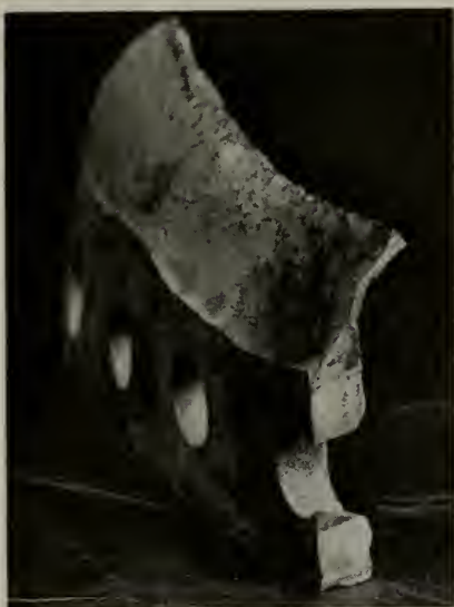
Figure 6—Parts of the lower drum of a water tube boiler showing the manner external corrosion wastes away the metal and weakens the head.
