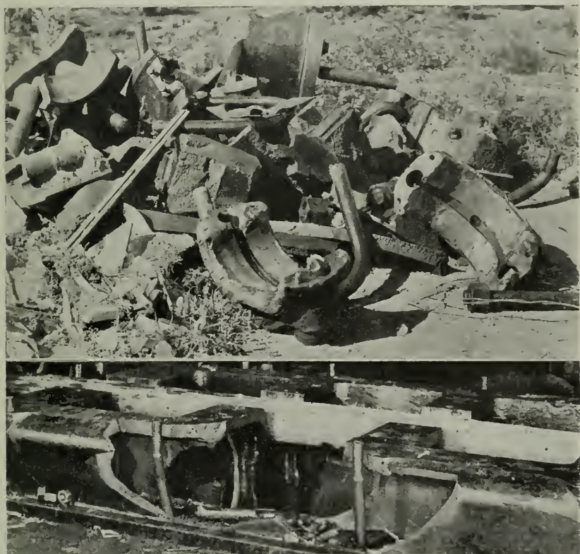
Figure 1—Above—This pile of metal contains parts of a 600 hp Diesel engine which was destroyed in a second or two when it over-speeded. Below—One side of the engine base after the broken engine parts passed through it.
