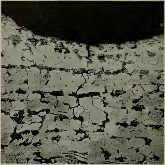
Figure 7—Embrittlement disintegration at 225 magnifications as produced in the laboratory.
