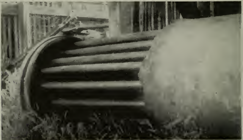
Figure 2—Condenser which exploded when poor girth seam welding permitted a 34" piece of plate to tear out.
