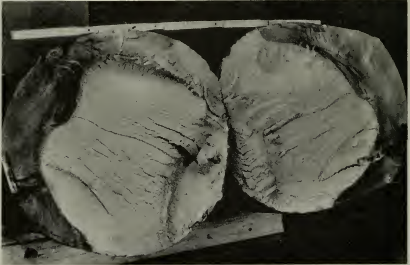
"The darker metal shows how far the crack has progressed."
