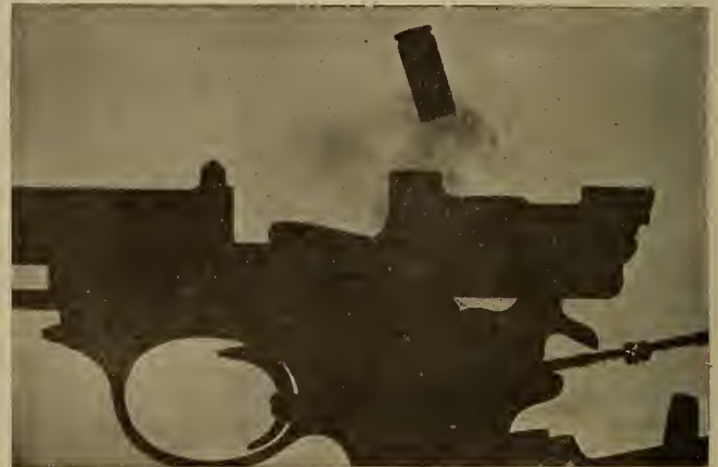
Fig. 7.—Showing Unconsumed Grains of Powder.
