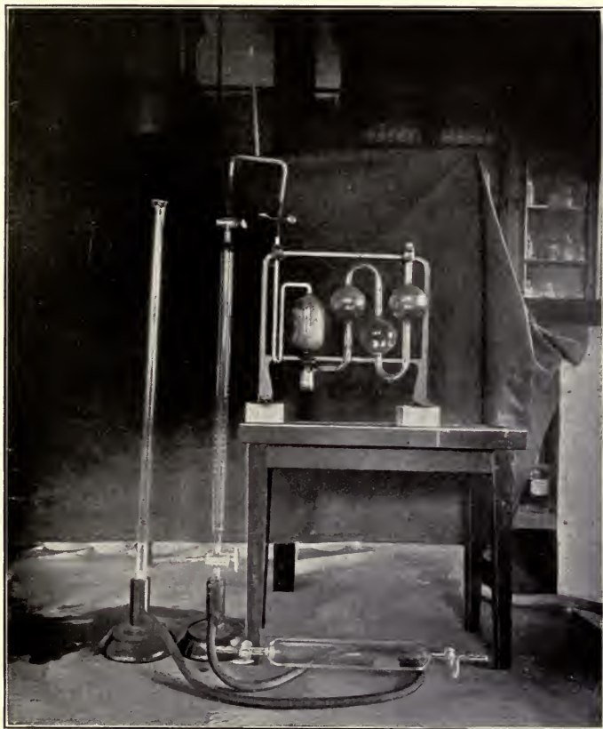
FIG. 26. Apparatus for determining the proportion of oxygen in air. The sample of air to be analyzed was collected in the receptacle which lies on the floor.
