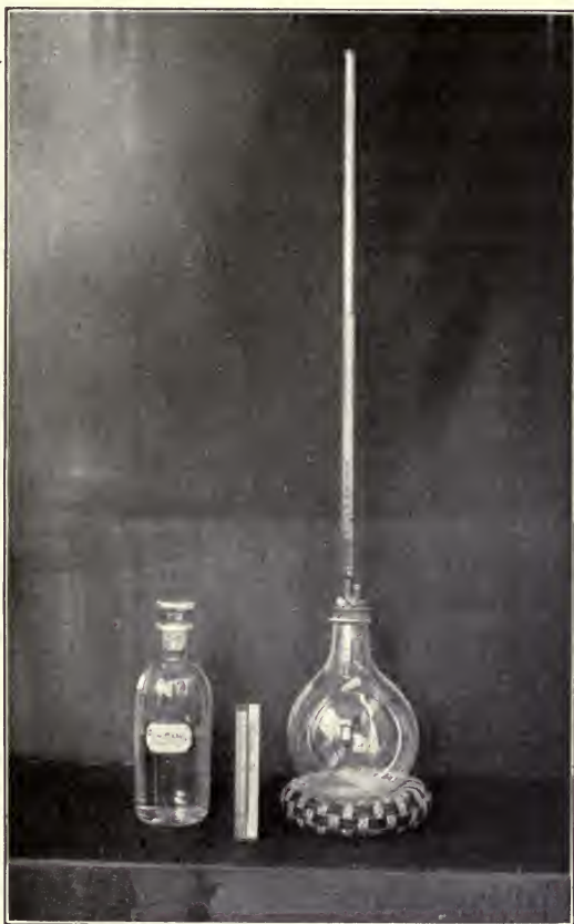
FIG. 24. Apparatus for carbon dioxide analyses. Method of titration with oxalic acid after the absorption of the carbon dioxide by barium hydroxide.
