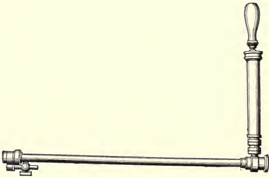
FIG. 39. Aitken's koniscope to determine the number of ultimate dust particles in air.
