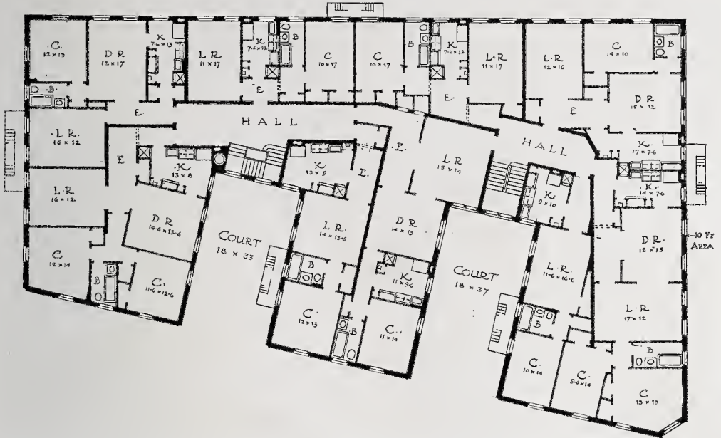
FIG. 75. TYPICAL FLOOR PLAN—GOLD MEDAL APARTMENT HOUSE, CORNER OF GRAND CONCOURSE AND 167TH STREET, NEW YORK CITY. Springsteen & Goldhammer, Architects.
