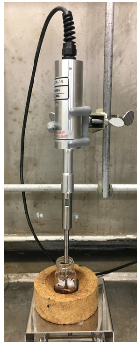
Figure 32. Ultrasonic Dispersion of BNNTs
