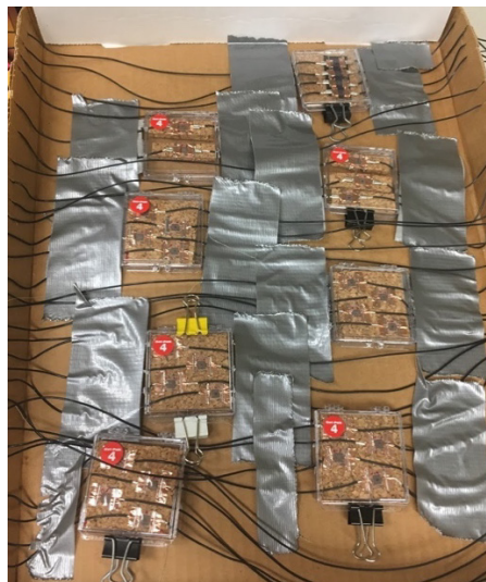
Figure 50. Array of Sensor Housings
