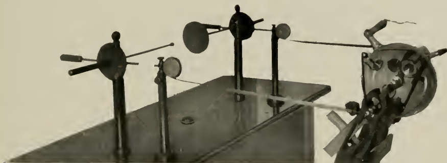
Fig. 49. The inverse spark gap on the left is open, on the right is closed.
