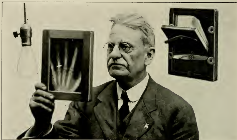
Fig. 77. Showing how the printing frame is held up to the light to expose the photographic paper. Also showing the back of the printing frame, the frame half open, and the photographic paper in position.
