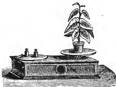
Fig. 51.—Balance for estimation of amount of transpiration. After Oels.
