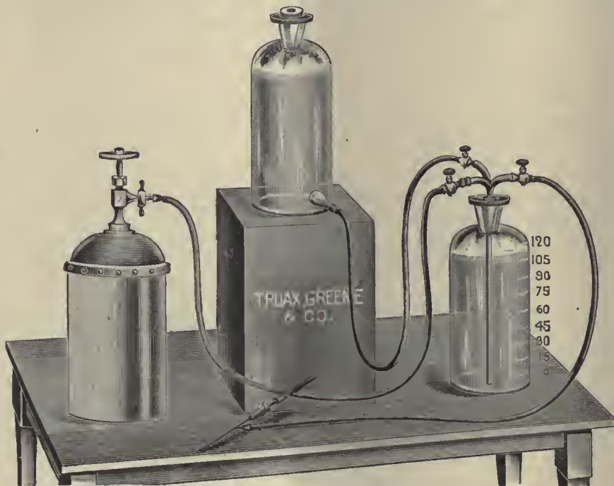
Apparatus for injection of the gas.
