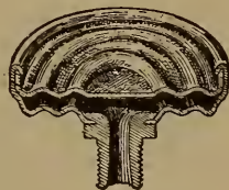
FIG. 22. Utica Capsular Spring.
