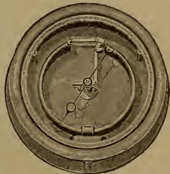
FIG. 13. Lane Pressure Gauge.
