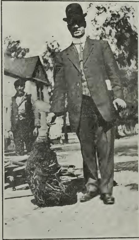
ROOT EXTRACTED FROM A SEWER IN CLEVELAND, OHIO
