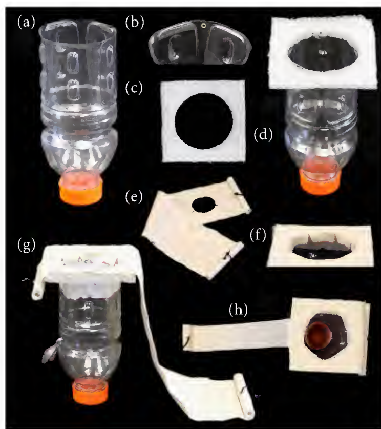
FIGURE 7: Bottle trap design: (a) inverted 600 mL plastic bottle, (b) hole bored into base of bottle, (c) foam square cut to bottle base, (d) foam square place around bottle base with fishing line tied through holes and around square, (e) canvas strip, with hole, slits around hole, dowels at each end, and zip-ties added, (f) canvas attached to inside of bottle with hot glue (g) fishing weight added to bottle with fishing line, and (h) excess canvas trimmed from foam square.
