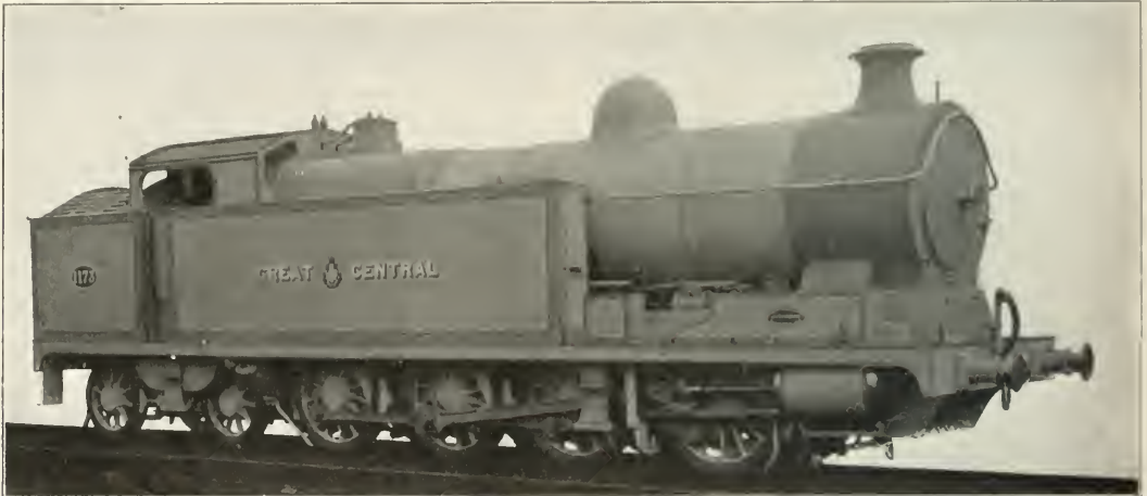
Heavy Tank Switching Locomotive for the Great Central Railway (England).
