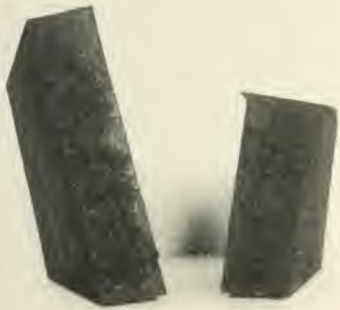
Burned Metal of Schoen Steel Wheel.
