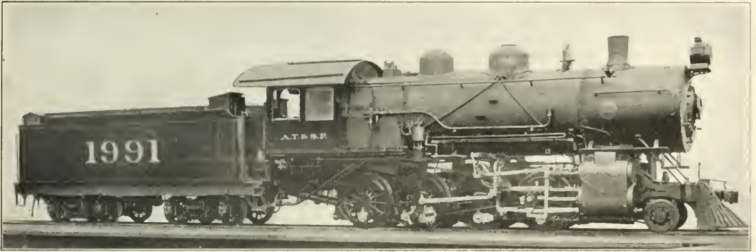
Consolidation Locomotive Built for Atchison, Topeka & Santa Fe, by Baldwin Locomotive Works.
