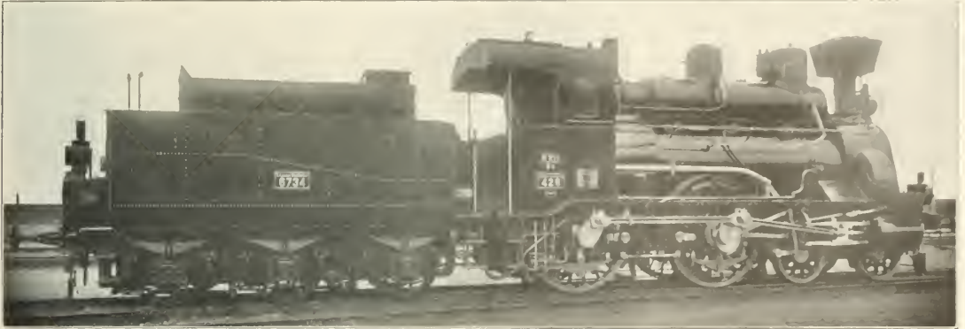
Passenger Locomotive for Austrian State Railroads, Fitted with Brotan Boiler.
