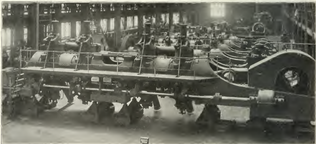
Westinghouse Horizontal Double-Acting Gas Engine.
