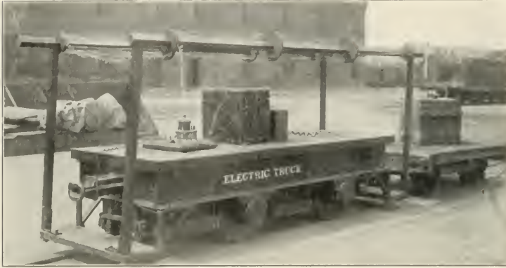
Wireless Controlled Electric Truck; Union Pacific.
