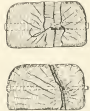
Fig. 11—Beech Ties with Wooden Dowels, Metal Clamps and Screws.
