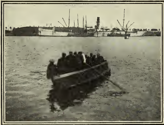
THE ENGELHARDT BOAT EXPANDED, WITH TWENTY-TWO MEN ON BOARD, TESTING ITS STABILITY.
