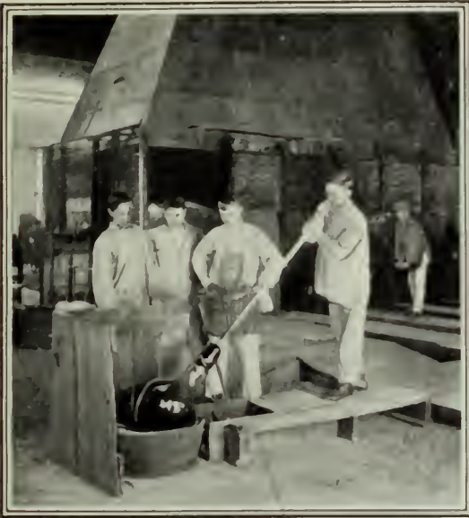
BLOWING THE BALL IS THE MANUFACTURE OF WINDOW GLASS.
