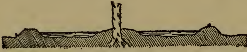
FIG. 48. Grading of interior of basins to prevent water from coming in contact with trees.
