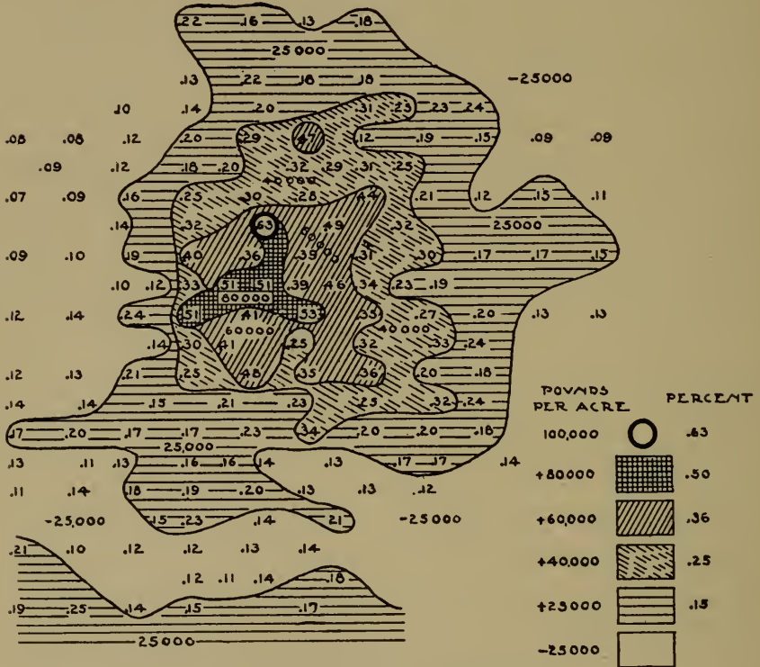
FIG. 113. Structure of an alkali spot.
