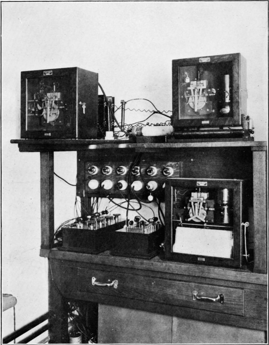
NEW RESPIRATION CALORIMETER. AUTOMATIC DEVICES FOR CONTROLLING TEMPERATURES AND RECORDING TEMPERATURE DIFFERENCES.
