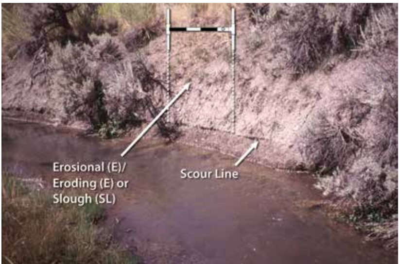
Figure 10. The streambank has an obvious scour line. The bank evaluated is above the scour line to the first bench and is recorded as erosional (E) and slough (SL) or erosional if the bank angle is within 10 degrees of vertical (Burton et al. 2011).
