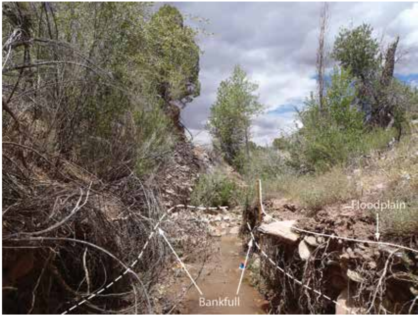
Figure D4. Location of bankfull and floodplain heights. Bankfull and floodplain heights differ when no flat depositional feature exists at bankfull height.
