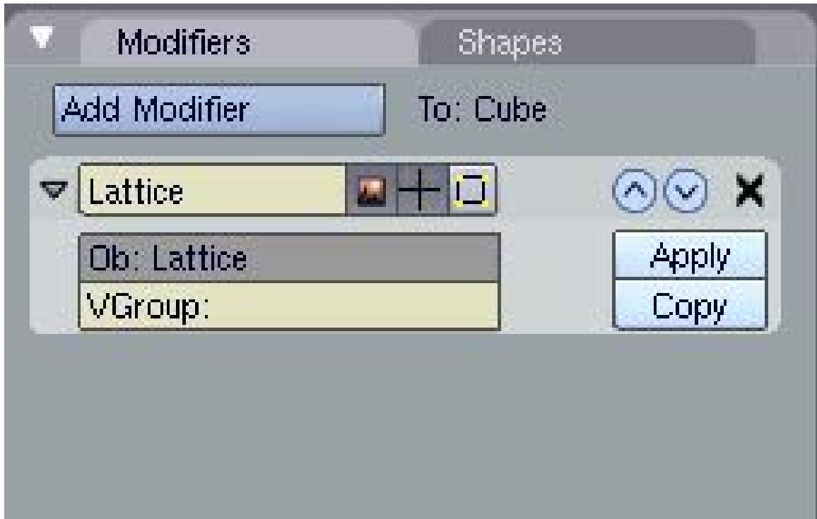
Figure 903 Adding a Lattice Modifier to an object
