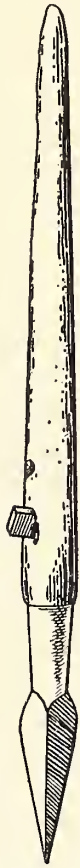
FIG. 3.—Hand pick used for making sockets in gravelly bottom for insertion of shibi.
