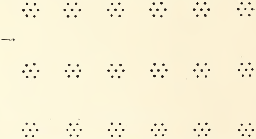
FIG. 22.—Arrangement similar to fig. 20, but adapted to rapid current, rows of collectors separated by intervals of 8 or 10 feet.
