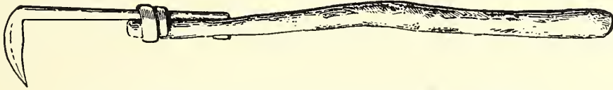
FIG. 13.—Oyster hook used for dislodging well-grown oysters from the shibi.
