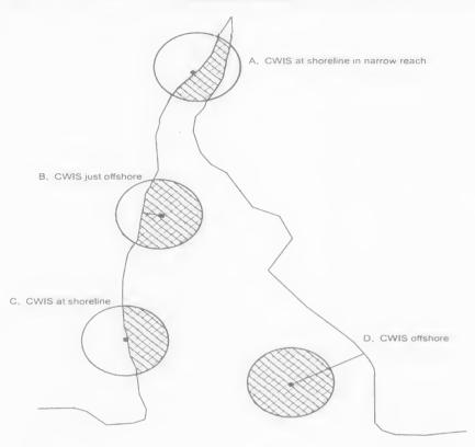
CWIS = Cooling Water Intake Structure
