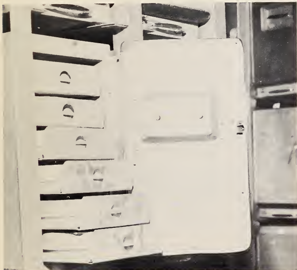
Electrically heated oven keeps food hot until delivered to aircraft.
