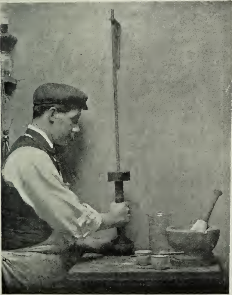
Grinding Enamel in an agate mortar, with a pestle attached to a rod passing through a hole in a bracket, and loaded with a lead weight.
