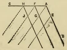
at which the lines meet will be the correct place to put the stake G; then proceeding, let one of the lines be brought to G, the other to H, and insert a stake at the point of meeting, I. If this is done carefully it will be found that the stakes all range most beautifully, no matter from where viewed, and on almost any shape of ground.
