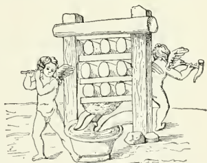
Fig. 159.—Oil press. From a wall painting found at Herculaneum.
