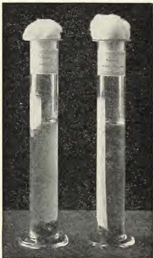
FIG. 32.—Decomposition of cellulose in solution (left) repeatedly changed, or (right) not changed.
