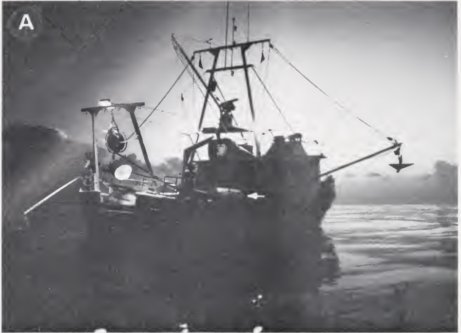
FIGURE 1. Capture and transport. A. R/V ERIN LEDDY-JONES nightlighting for Loligo plei off the coast of Galveston, Texas in 17 m of water. Note the 1000-watt quartz-iodide lamp on the A-frame and two 500-watt quartz-iodide lamps amidships that are used to attract squids. Squids are dipnetted on board (left) and placed in a transport container (arrow). B. Three types of transport containers: VT is the vertical tank; HCT is the horizontal cylindrical tank; RHT is the rectangular horizontal tank. The tanks and squids are all drawn to the same scale. The squids equal the approximate size of 200 mm mantle length. Water flow is indicated by arrows. In the RHT, (A) is the removable partition that is replaced when approximately 15 adult Loligo spp. are put in the tank. The tank top (B) is then secured with stainless steel bolts (C) that force a rubber gasket (D) against the top edge of the tank, producing a water-tight seal. Another 15 squids are placed in the upper compartment through the chimney (E). When water quality is good, sea water is continually pumped into the base of the tank through (F) and allowed to overflow from the chimney. When water quality deteriorates near shore, the tank water is circulated by a submersible pump (G) that pushes the water through an exterior filter (H) and back into the tank. Pure oxygen or air may be added through a valve (I).
