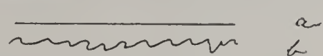
(a). Line drawn by the fixed pencil, (b). Sound-curve transmitted by the diaphragm.
