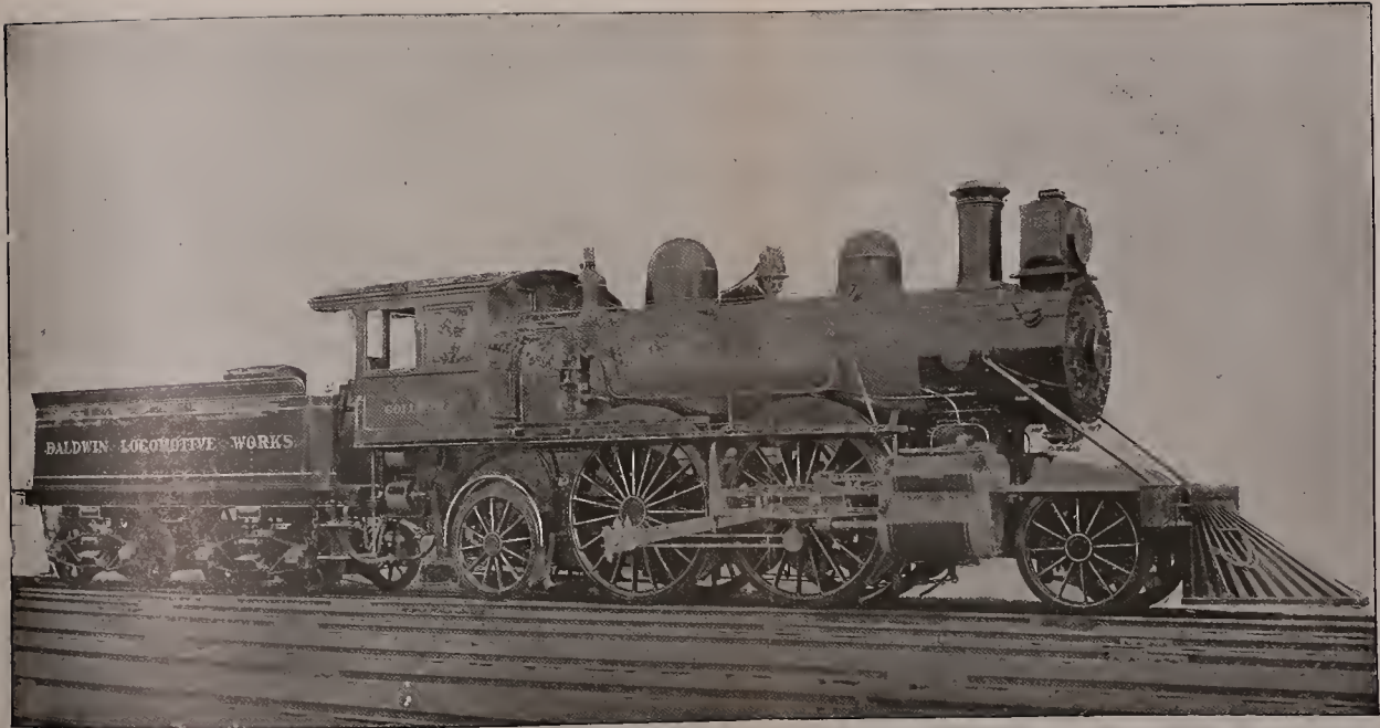
PLATE IX.—Compound Express Passenger Engine, “Special High Speed” Type, No. 13,350. Built by Baldwin Locomotive Works.
