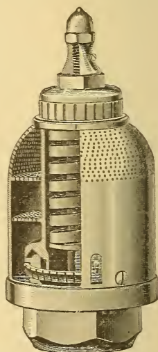
Fig. 49. Meady Muffled Locomotive Pop Safety-valve.
