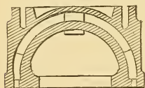
Fig. 80. Allen Balanced Valve, Pennsylvania Railroad, Class "O." Lengthwise Vertical Section to one side of Centre.
