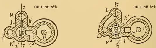
Figs. 165 and 166. Sections of Schenectady Compounds.
