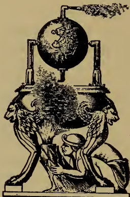
FIG. 460. Hero's Reaction Turbine.
