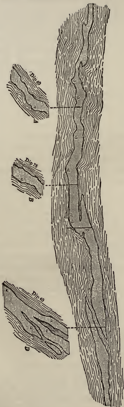
Fig. 28.—A horizontal section, with transverse vertical sections of a typical mica "vein" at the Presnel mine, Yancey County, North Carolina.
