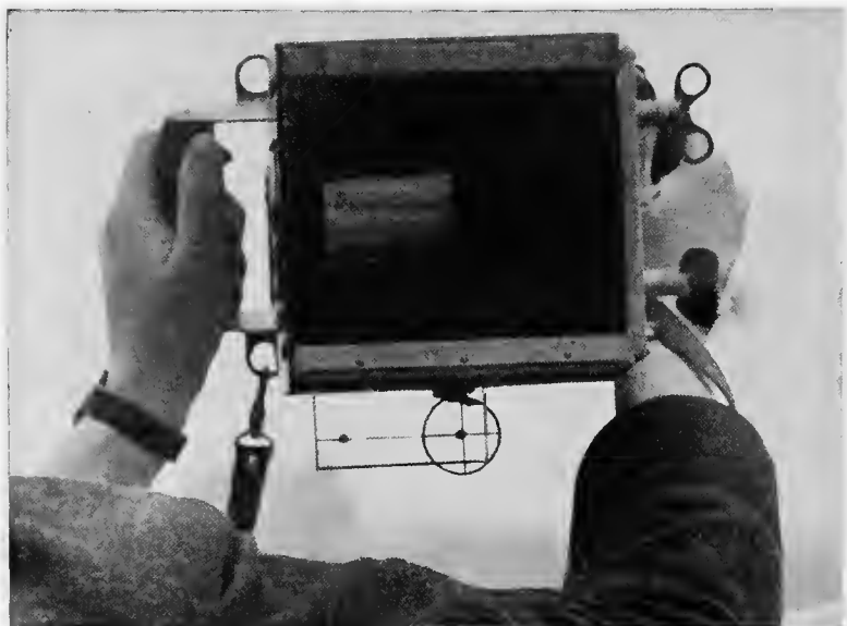
Fig. 157.—Aerial hand camera fitted with two complementary shutter slits and double sight, for stereoscopic photography.
