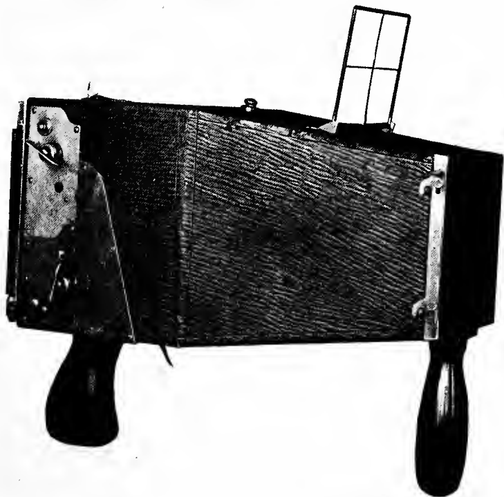
FIG. 37.—Pistol-grip aerial hand camera.
