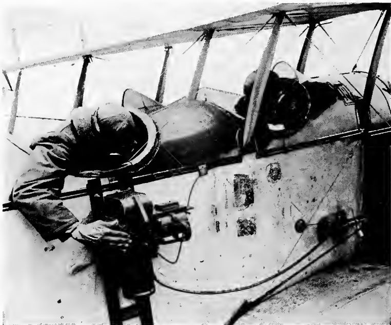
FIG. 81.—“L” camera mounted outside the fuselage. Observer using exposure plunger, pilot using Bowden wire release.
