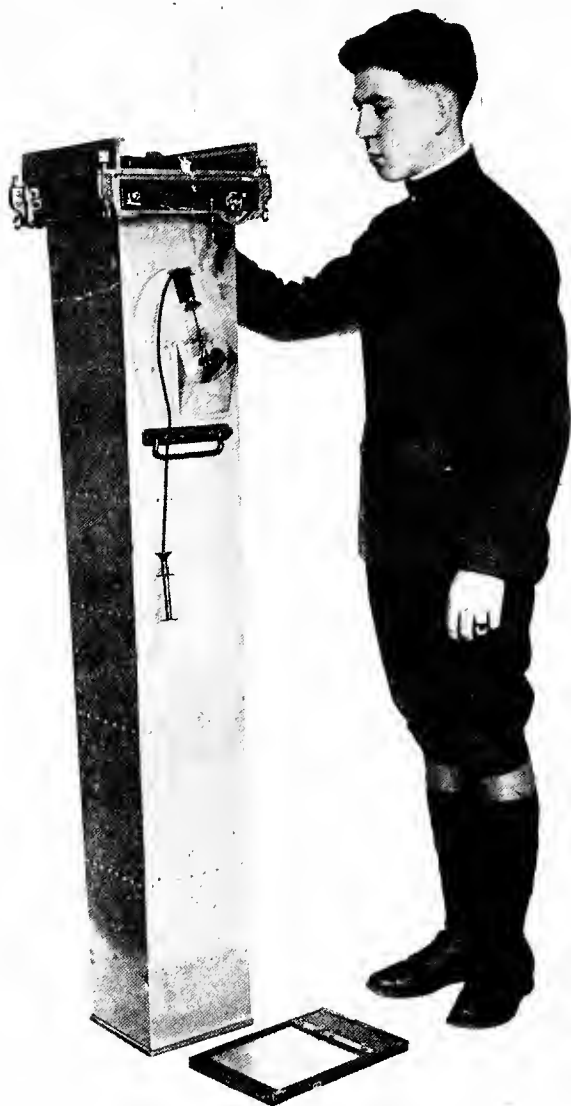
FIG. 41.—120 centimeter deMaria camera.
