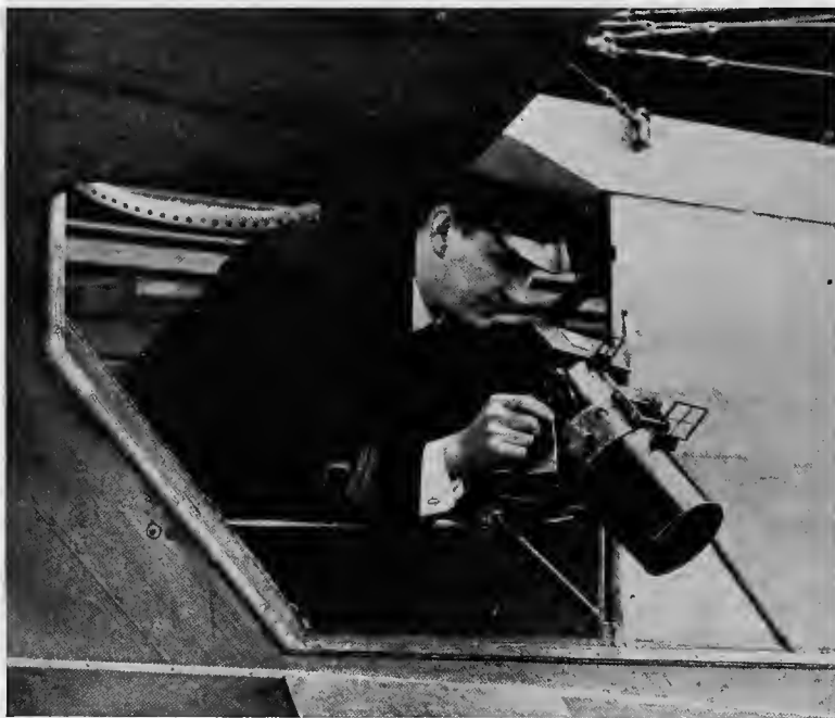
FIG. 185.—English "Type 18" hand camera on bracket for exposing through side window of flying boat. British official photograph.
