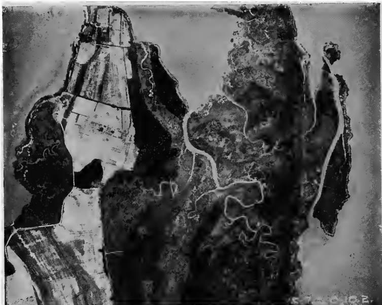
FIG. 200.—An aerial photographic survey of ground difficult to cover by ordinary surveying methods.
