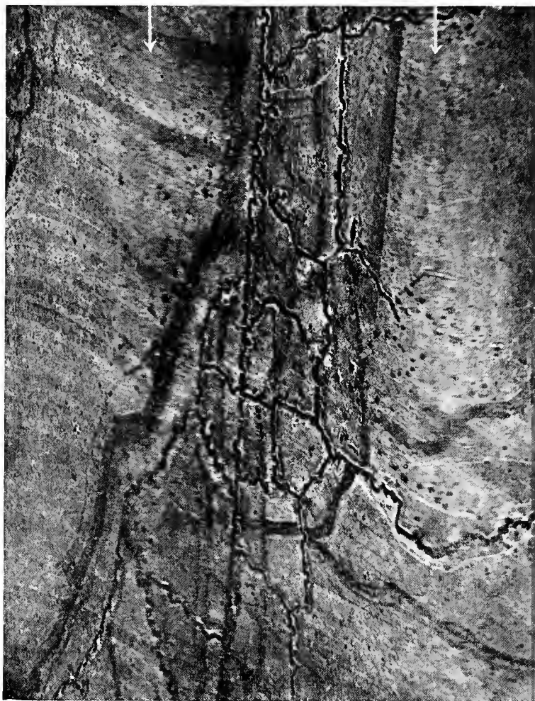
FIG. 76.—Captured German photograph, showing zones of poor definition due to vibration during passage of focal plane shutter aperture.
