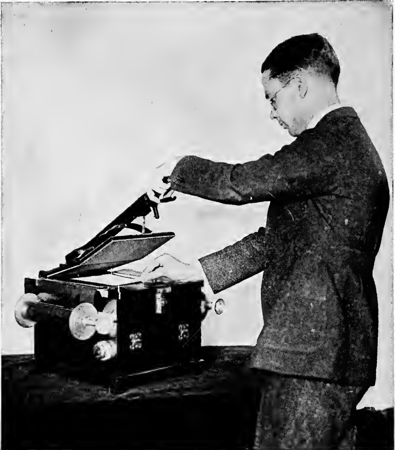
FIG. 120.—Film printing machine.
