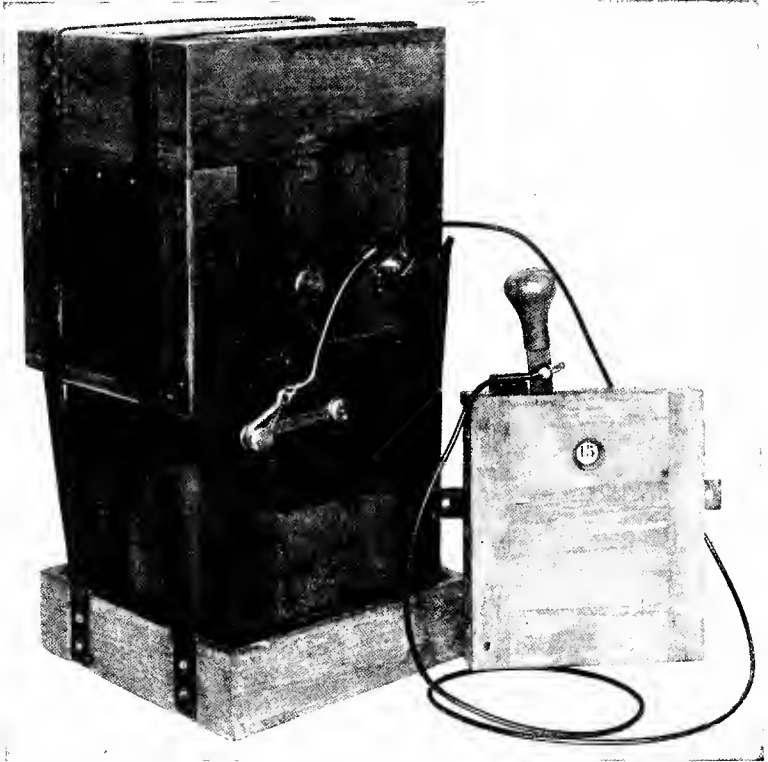
FIG. 49.—Italian (Lamperti) single-motion plate camera, on anti-vibration tray.
