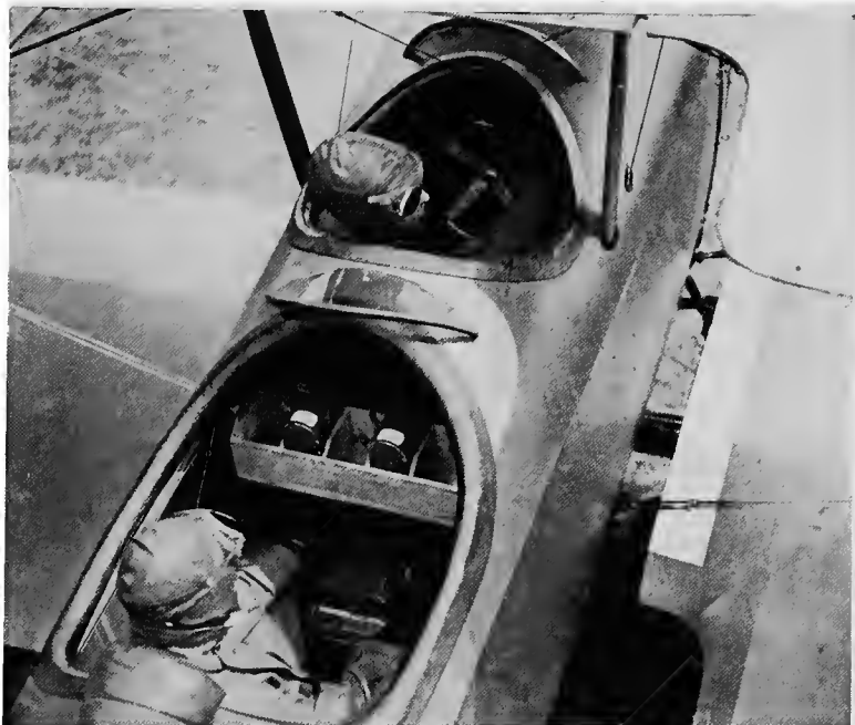
FIG. 36.—Training plane equipped for photography, showing "L" camera in floor mount and magazine rack forward of the observer.
