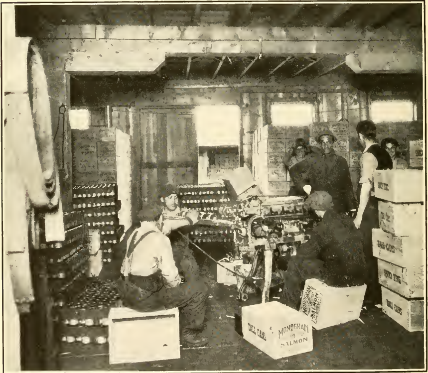
FIG. 34.—SALMON CAN-LABELING MACHINE.
