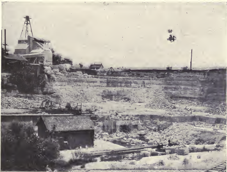
PLATE VI, FIG. 2. — General view of a limestone quarry, showing stratified character of the rock.
