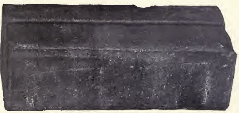
PLATE XLIX, Fig. 2. — Repressed brick. The rounded edges and corners as well as the grooves were produced in the repressing.
