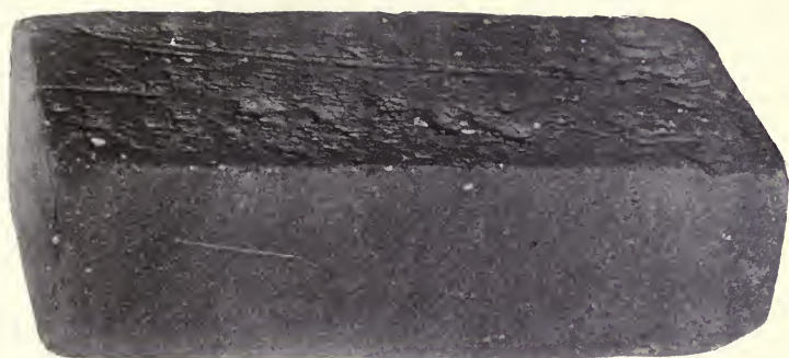
PLATE XLVI, Fig. 1. — Common red soft-mud brick. The roughness of upper surface is due to striking off excess of clay in mold. The other two exposed surfaces are sanded ones.
