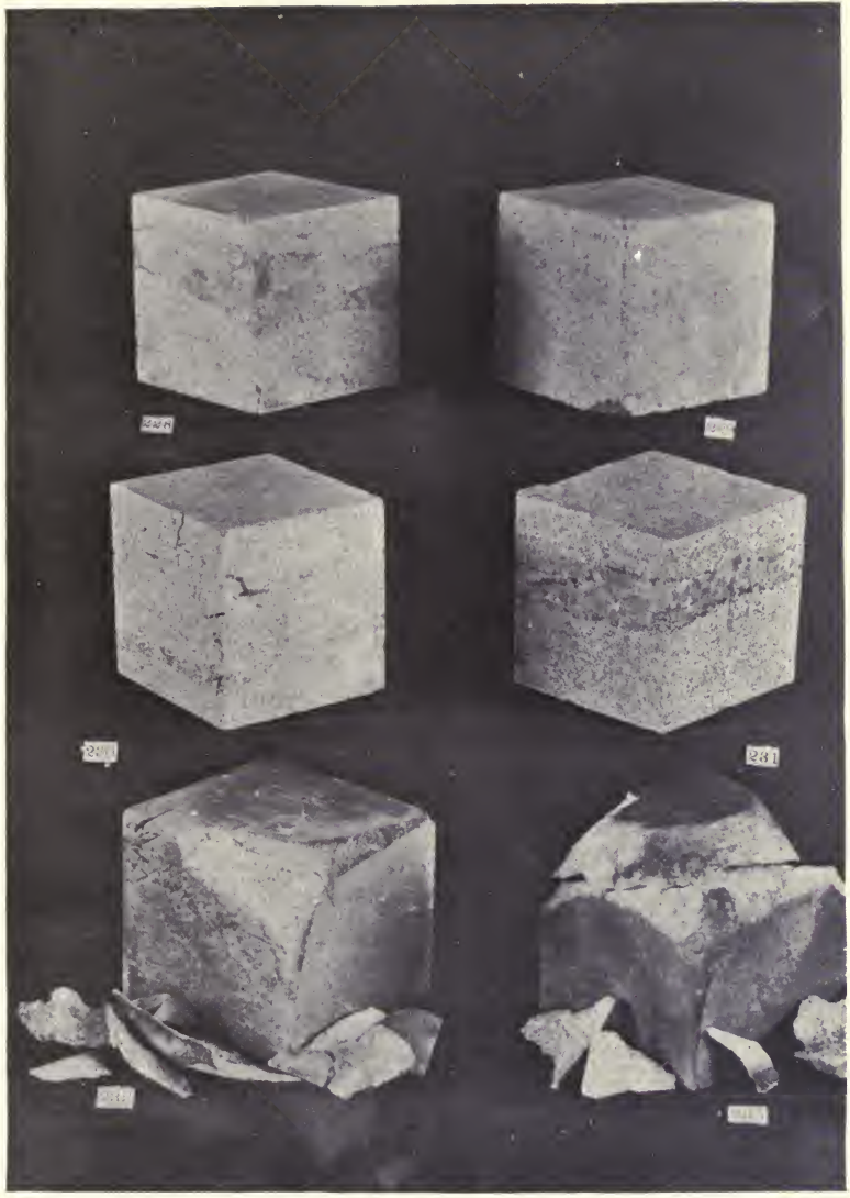
PLATE XIII. — Fire tests of 3 inch cubes of gneiss, Mt. Arlington, N. J. (After W. E. McCourt.)
