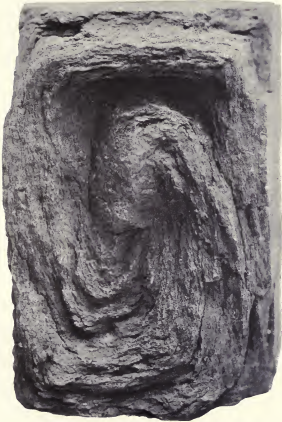
Plate XLVII. — Section of stiff-mud brick showing laminations.
