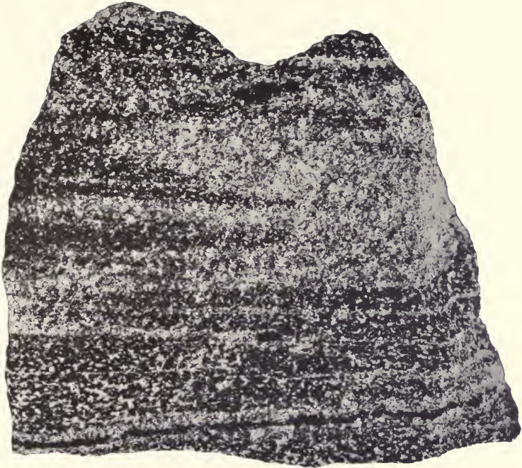
PLATE VII. — Biotite gneiss, showing characteristic banded structure of this rock.
