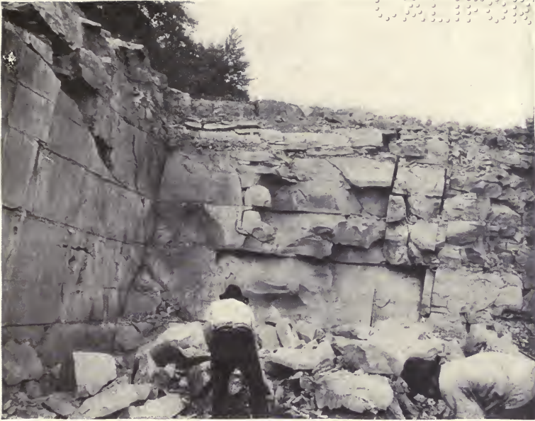
PLATE VI, FIG. 1. — View in a limestone quarry, showing the horizontal stratification planes and vertical joint planes. (H. Ries, photo.)
