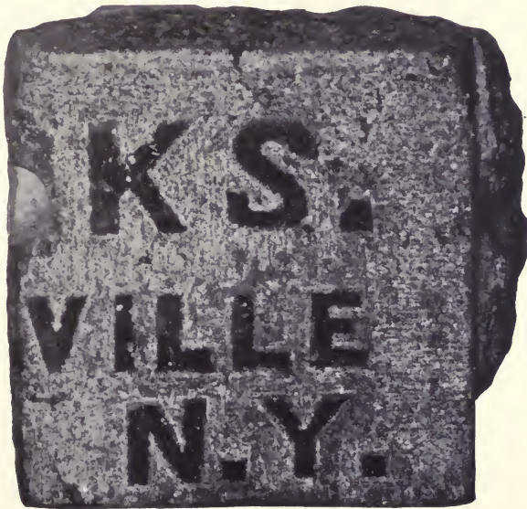
PLATE VIII, Fig. 2. — Gabbro from Keeseville, N. Y., showing contrast between tooled and polished surface.
