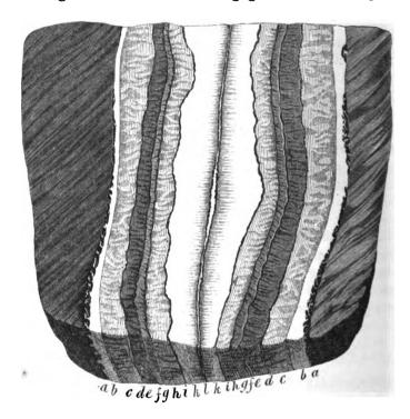
minerals are:—a, blende; b, quartz; c, fluor-spar; d, a thin layer of detached crystals and particles of blende; e, irregular-curved crusts of heavy-spar; f, a thin layer of white iron pyrites; g, heavy-spar; h, fluor-spar; i, white iron pyrites; k, white calc-spar; l, pale yellow calc-spar, forming small druses at some parts of the middle of the lode.
