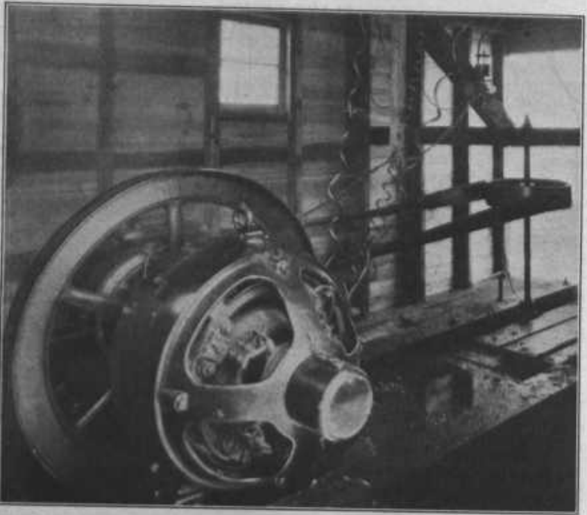
FIGURE 9.—Quarter-twist belt drive from a 26 by 6 inch pulley on the vertical shaft of a 15-inch turbine to a smaller pulley on the generator
