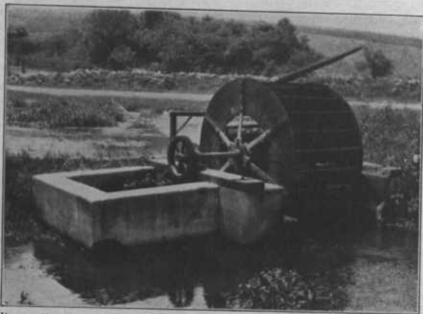
FIGURE 19.—Downstream side of a 5 by 3 foot undershot wheel geared to a 2½ by 4 inch triplex pump. The machinery cost $205 in 1914. Pennsylvania
