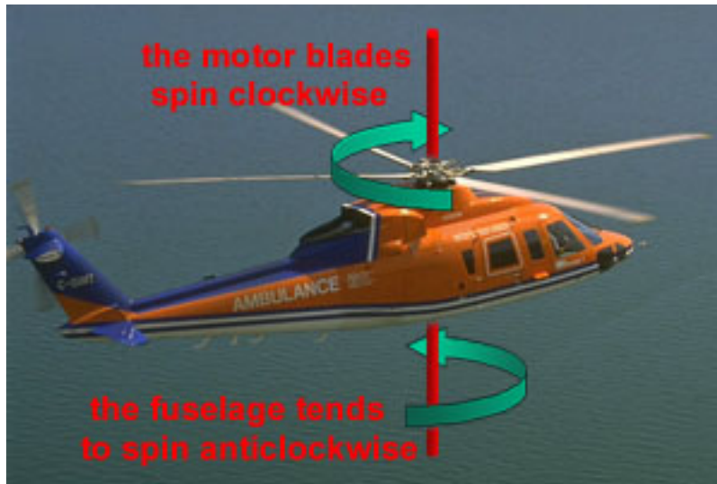
Figure 3. Illustrating the requirement for a tail rotor. From Ref. [http://www.phy.cuhk.edu.hk/phyworld/iq/helicopter/helicopter_e.html].
