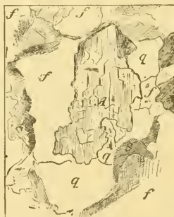
FIG. 2. Authigenetic augite in altered sandstone, No. 8 Coast Ranges. A , augité; u , uralite; f , microcrystalline feldspar; q , quartz grain; s , serpentine. Magnified 117 diameters.
