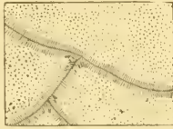
FIG. 9. Serpentine forming from sandstone and composed of fibers normal to the attacked surfaces.
