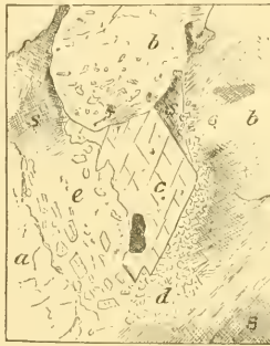
FIG. 3. Authigenetic hornblende in altered sandstone, No. 8, Coast Ranges. a , clastic quartz; b , clastic feldspar; c , authigenetic hornblende; d , authigenetic feldspar aggregate; e , clear isotropic mass; f , serpentine. Magnified 170 diameters.
