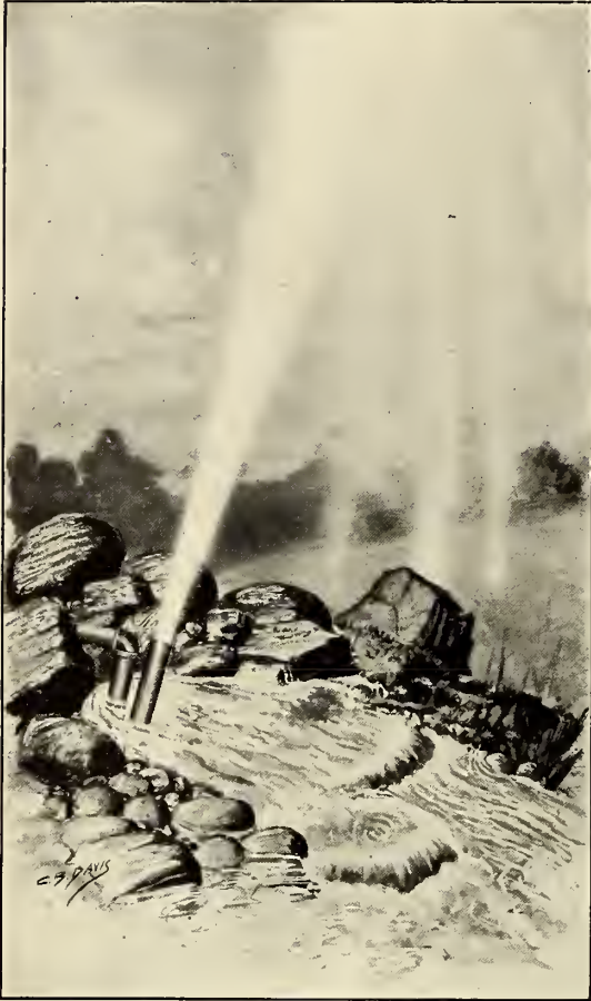
THE OUTSIDE END OF THE BLOW-OFF PIPE (J).
