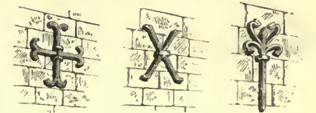
Medieval Tie-rod Anchors. (From Viollet-le-Duc's "Dict. de l'Architecture.")
