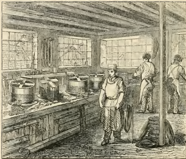
COARSE WIRE DRAWING.
