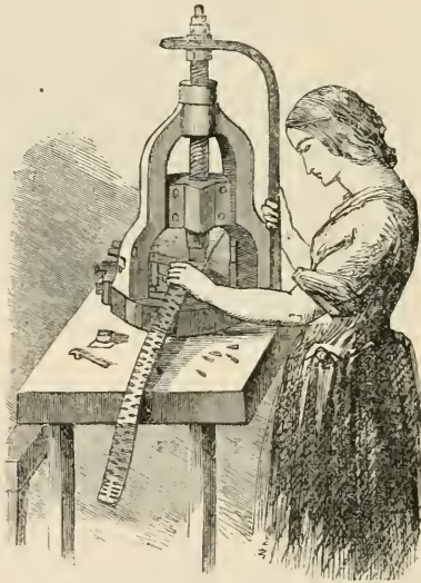
STAMPING THE PEN FROM THE STEEL.
