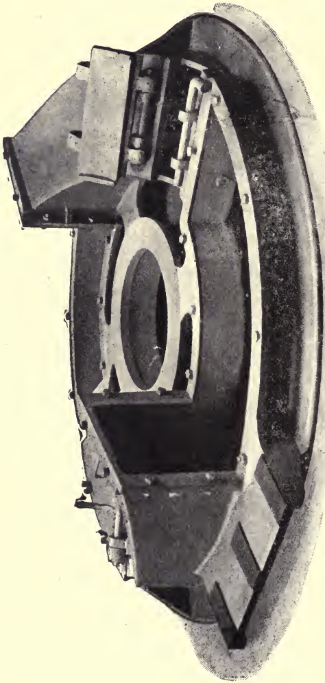
FIG. 23.—Beet-slicing machine showing foundation parts or body of machine.
