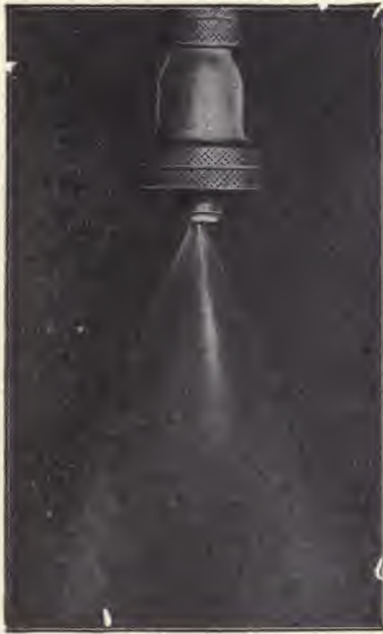
FIG. 180.—Injector for use in maceration of megass (KESTNER).
